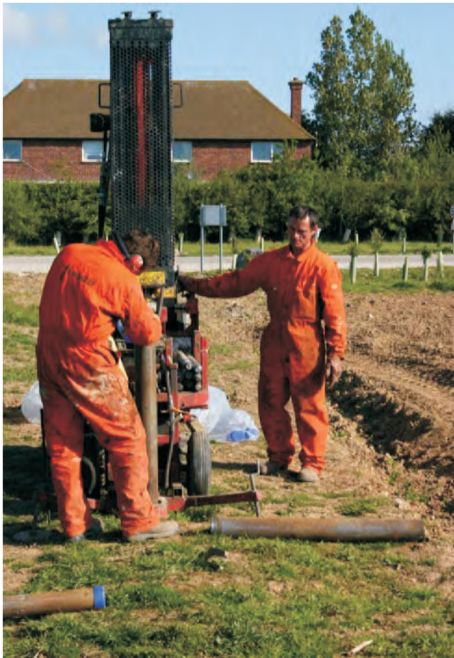
Fig 37 A Terrier rig recovers 1m long core samples which are then logged (Bates 2005a)
